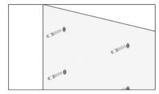
Put the expansion tubes into the holes.
