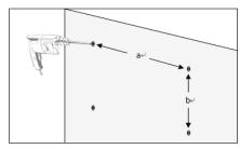
1. Drill the holes on the wall, make sure the positions are correct.
