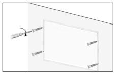
3. Insert the screws through the mounting holes on the front panel, then screw into the tubes.
